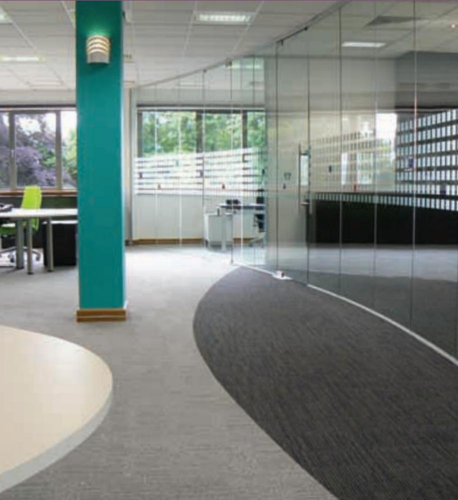
Available in either straight striking lines, faceted or the most graceful curves, Polar single glazed minimalist form is designed with the minimum of components, thus facilitating speed of erection without compromising structural stability and rigidity. The patented bubble joint ensures a virtually frameless system with no vertical posts between modules, corners or three way junctions.
