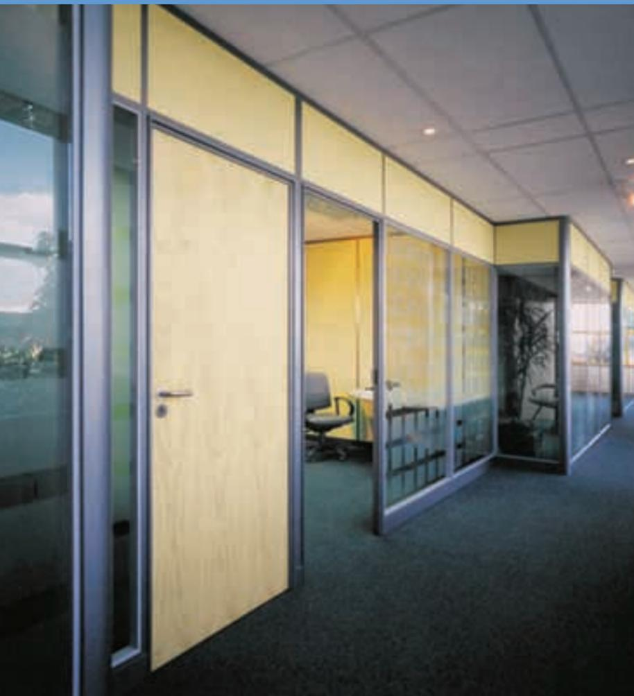
The system has been tested for sound attenuation and achieves up to 40dB (Rw) in double glazed format.
