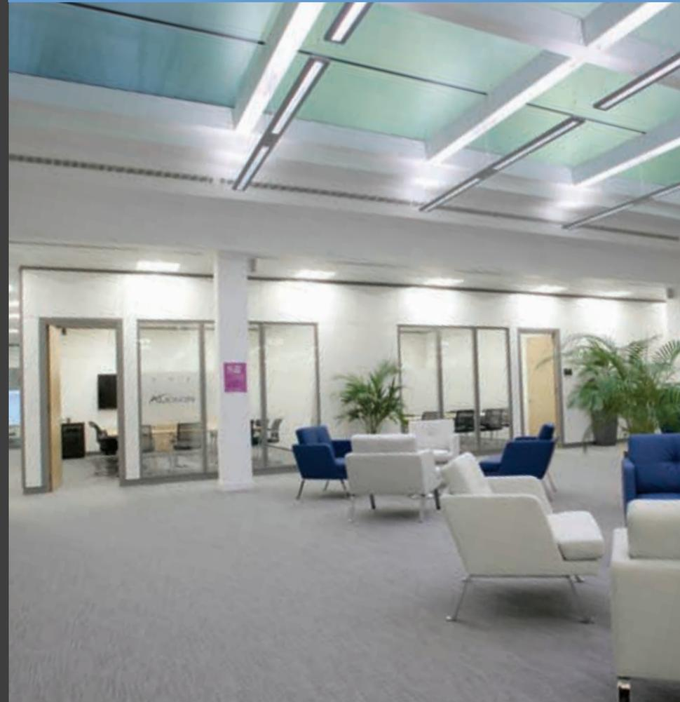
Panel modules are interchangeable from glass, veneered, fabric or metal panels without disturbance to adjacent components. Its hung panel design, with recessed base and head, creates a true floating panel effect with no visible framing on solid elements.
